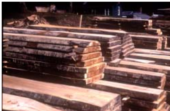
Top : Front of the workshops at Ancrum Middle : Oak in the round ready for the saw Bottom : Beech and elm air drying in the yard
